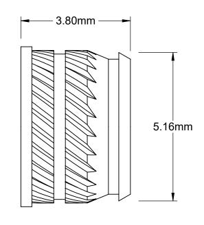
For Minimum Material Thickness: 4.57mm For Maximum Hole Diameter: 0.199in
