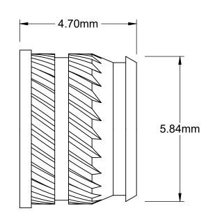
For Minimum Material Thickness: 5.47mm For Maximum Hole Diameter: 0.226in
