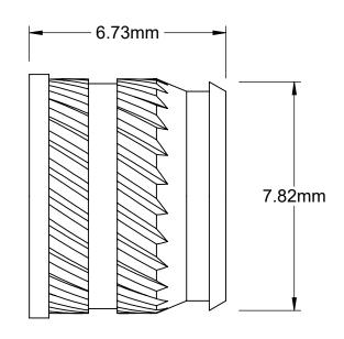
For Minimum Material Thickness: 7.50mm For Maximum Hole Diameter: 0.303in
