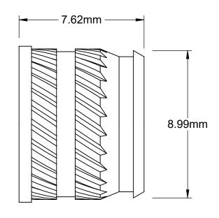
For Minimum Material Thickness: 8.39mm For Maximum Hole Diameter: 0.349in
